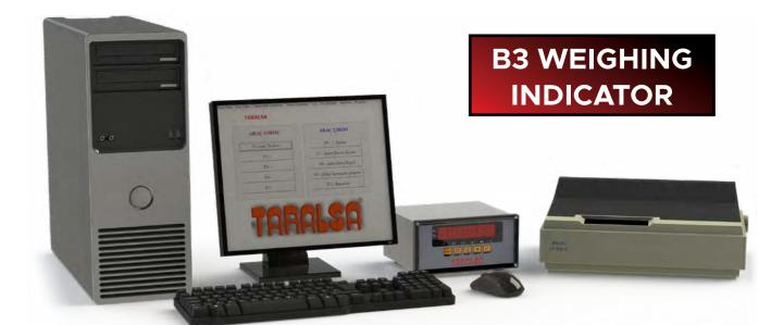
The B3 series weighing indicator is basically a desktop type for weighing applications. 6 digits bright red led indicator, standard USB and serial communication interface exist on the indicator used in standard truck and lorry weighing applications. There is a lightning protection at the load cell input. Indicator has the ability to work smoothly in all industrial environments with its IP 54 protection class stainless steel structure.
